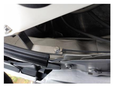
Connect the power wire beneath the nut on the power cable terminal on the driver's side strut tower.
