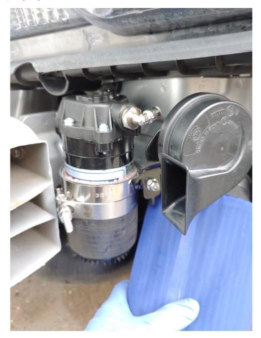
Remove horn and its bracket, unplug and set aside for now. The U shaped bracket will mount to the frame securing the clamp inside it, while the pump slips through the clamp itself; there's adjustability there to slide the pump up and down to get the pump in the position you want it.
