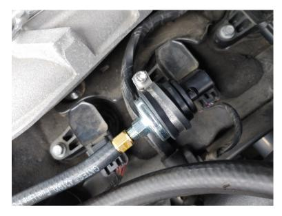
Tie the pressure switch into the BOV vacuum line. Use the included T fitting and hosing to tee into the BOV line and run to the barb fitting on the pressure switch.
