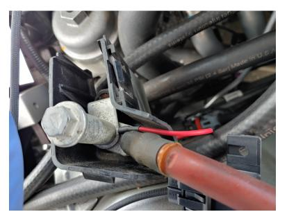
Back in the fenderwell, plug in the pump. The longest section of wire, run it over the engine in a neat fashion to the pressure switch; unplug the coil terminal closest to the pressure switch you mounted, plug the inline connection but leave the connector for the pressure switch unplugged for the moment, you'll plug it in to complete the install after we prime the system.
