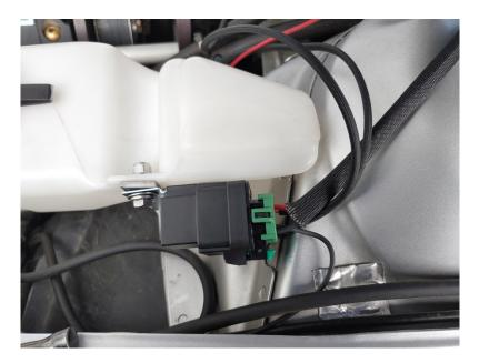
Connect the ground black wire to where the Z-angled reservoir bracket attaches to the fender above the headlight (remember there used to be a ground stud there from factory).
