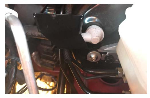
You'll need to use the new fluid reservoir as a guide as you bend the A/C lines out of the way. Use light to moderate pressure and push the lines over to make room for the new reservoir. Once space is created, the reservoir will sit right beside the brake fluid reservoir like this...
