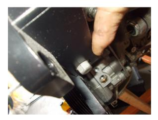
Firstly, torque the long M12 countersunk screw to 40 ft-lbs. Next, torque together the countersunk screw holding the two piece engine plates together to 15 ft-lbs. Lastly, torque the 15mm bolt to 20 ft-lbs.
