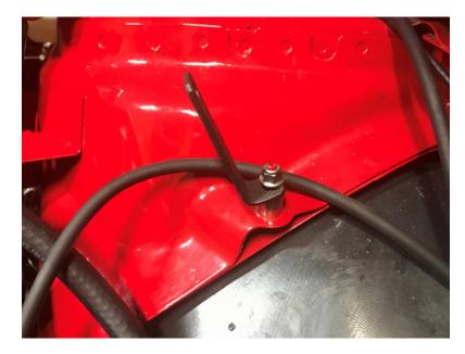
Install the included pump upside down so it sticks downwards. Use some lubrication on the rubber seal as needed and push the pump in fully to secure.
