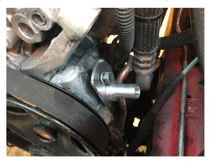
Next, mount the bracket for mounting the new fluid reservoir. Go back to the brake master cylinder; from the engine side, remove the nut securing the master cylinder to the brake booster. Slide the new bracket inplace over the stud, and note the two forks fitting around the casting to prevent the bracket from rotating. Reinstall the nut.
