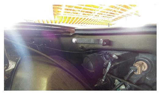
Next take the shorter bracket, spacer, and one of the nuts. This goes on the airbox stud on the strut tower. Slide the spacer on the stud first, then short leg of bracket, and nut.
