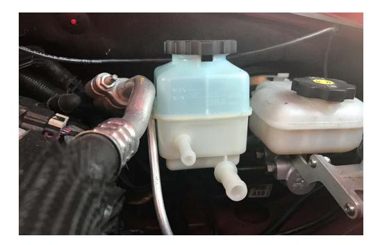
Install the large return hose onto the fitting using the short 90\* bend end. Ensure to angle the hose upward and prevent any low spots in the hose between the fitting and reservoir. Slide one of the hose clamps on and secure when happy with the positioning. Then trim the hose to length at the reservoir end using good scissors, razor blade, or a proper hose cutter, install a clamp, and secure to the reservoir.
