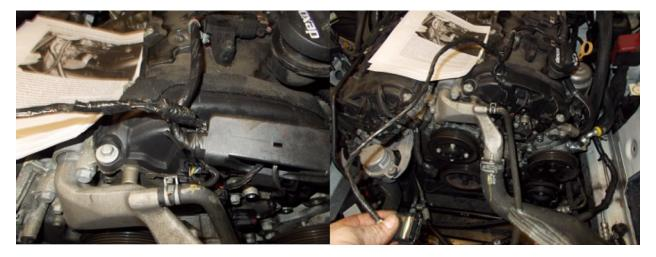
Once you're completed, tape the MAF wiring back up with new electrical tape, and clip the plastic retainer back into place.
